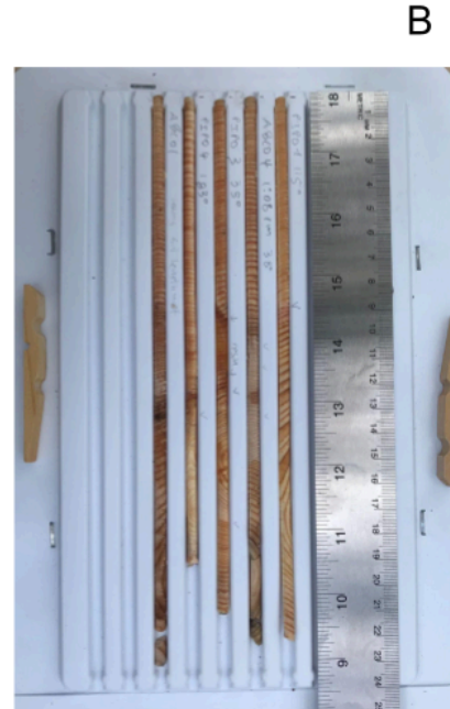
Figure 4 A) a screenshot of the webapp used to detect the sapwood depth. Note that the user clicks the start and end point of the core (white circles in thermal image) and enters the core length. This is used to determine which temperature values are sampled from the image, and their position along the core. B) A reference photo taken of the same cores. This is helpful for determining the presence and position of rot and if the core passed through the center of the tree.
