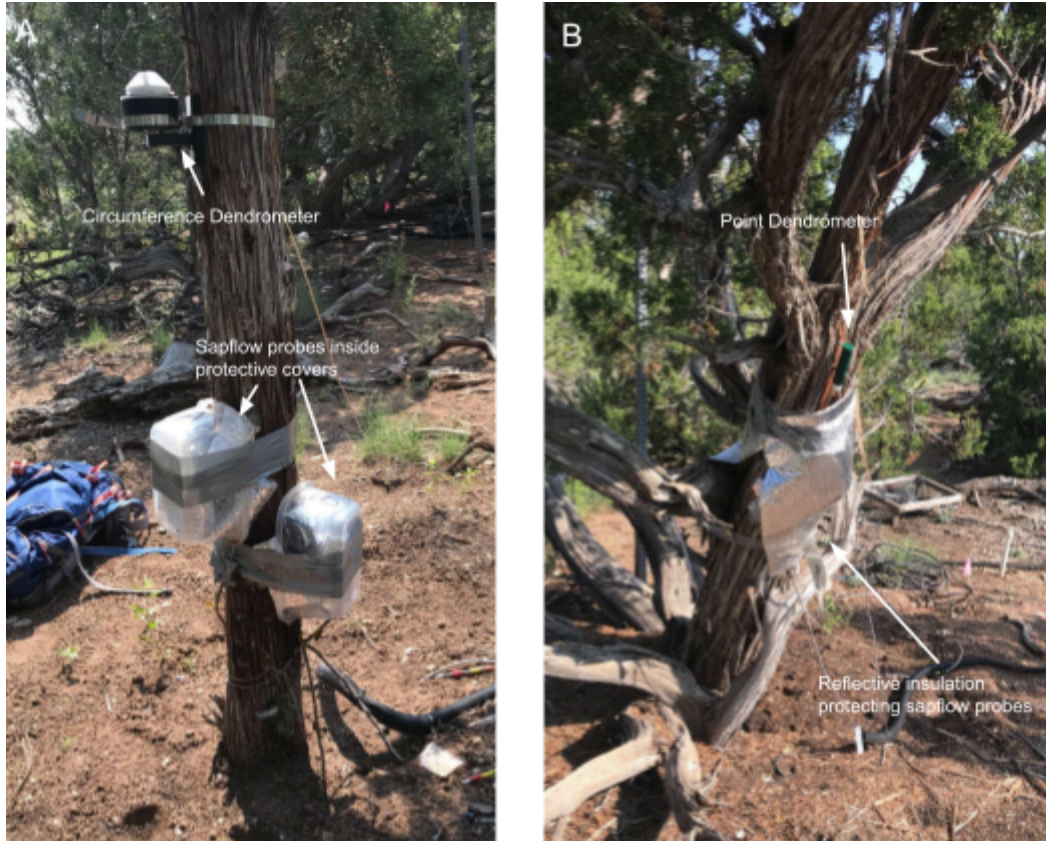
Figure 5 A: Circumference Dendrometer installed on a single-stemmed juniper at US-Mpj. Probe insulation was removed in this photo to take measurements. B: a point dendrometer installed on a multi-stemmed juniper at US-Mpj. Reflective insulation protects the sapflow probes from the sun.
